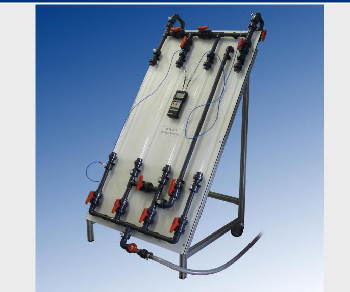
The "Flow networks" equipment reflects in scale the problem that usually appears for the calculation of pressures and flows in pipes that interconnect each other. These pipes usually have different diameters and lengths and form different systems (serial, parallel, mesh ...) which severely complicates the calculation.
